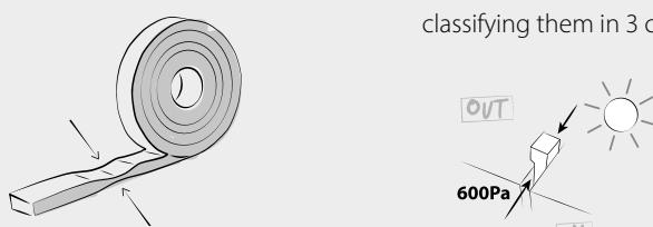
Products generally obtained from expanded polyurethane foam. Ideal for filling in irregular cracks that need to maintain high elasticity over time. Expansion times depend on the operating temperature at the worksite. Excellent thermal/acoustic insulation, permeability to vapour and heavy rain can vary.
