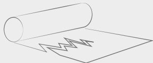
Force exercised both longitudinally and transversally, to determine the maximum load, expressed as N/50 mm.
